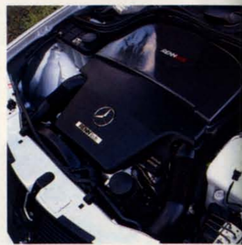
The stock 4.3-liter V-8 is transformed into a 6.0-liter 408-horsepower velvet brute. A six-speed shifter takes center stage in the carbon-fiber-enshrouded interior.
